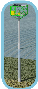
Above: Single Caisson Structure Below: Minimal Satellite Structure (Courtesy of Martec Limited)
