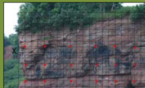
Figure 5: Lidar grid projection, scanning point selection and X-Y axes geometry
